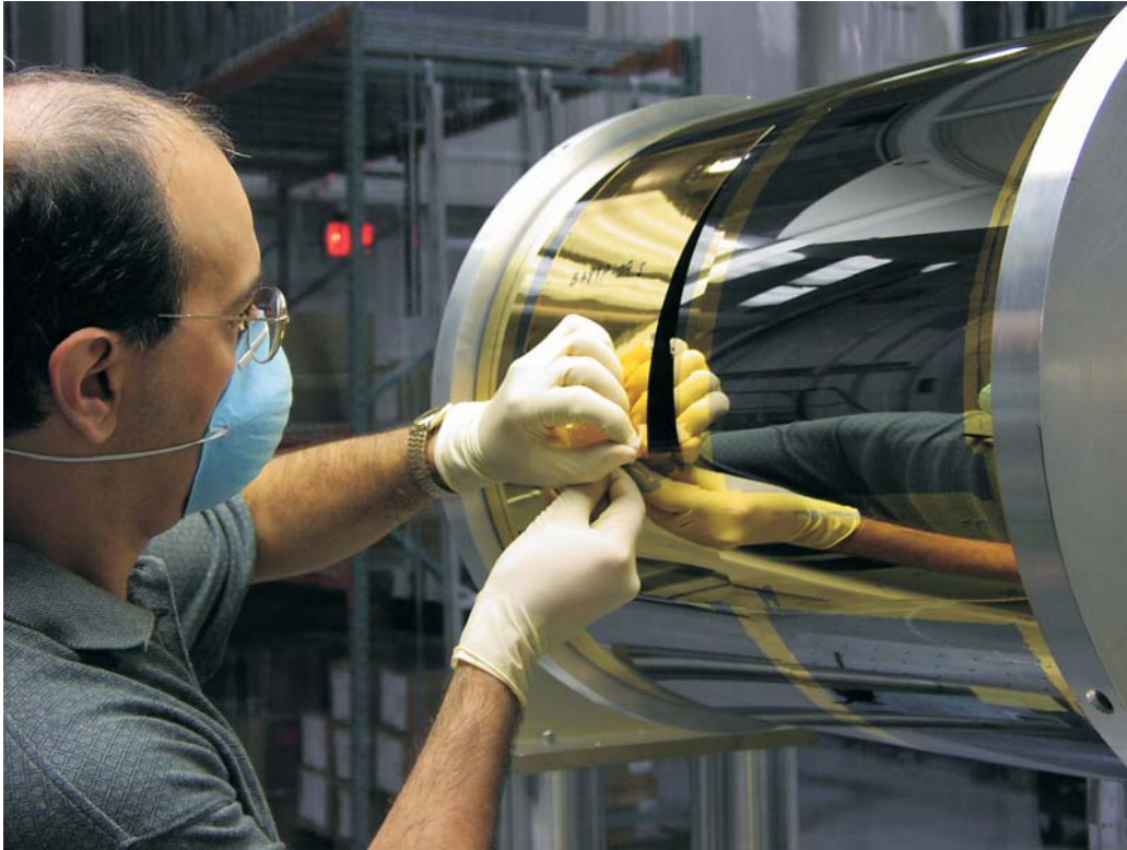
A prototype mirror segment for Constellation-X being separated from the replication mandrel.
